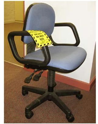
Chair with broken gas lift tagged out
