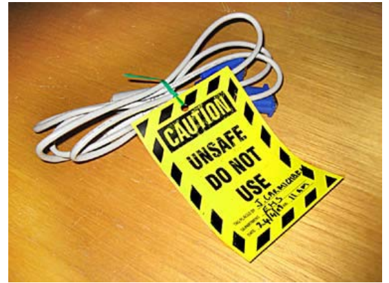
Damaged electrical cable tagged out
