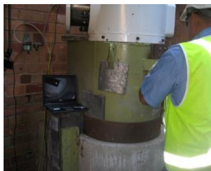
Using fibre optics to view the ^{60}\text{Co} from inside the vessel
